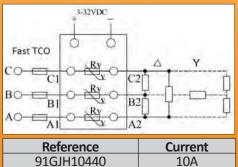
91GJH30440 30A Electromagnetic contactors and relays: see page 85
